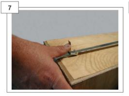
Hold stub of band with thumb and bend it over buckle.
