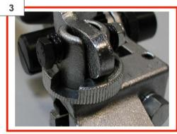
Before rolling over the tool over the buckle, it's very important to turn the knurled ring as shown in figure 3 + 4!
