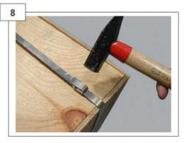
Hammer stub of band flat over bridge of buckle. Complete the clamp by hammering down ears over stub.
