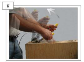
Pull on long handle with left hand, band is cut off to correct length. Then move tool forward and away from the buckle.
