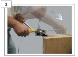
Place band in the nose of tool and ratchet slots. Hold short handle in right hand and push long handle forward in full arc with the left hand. This tightens the strap. When required tension has been applied, bring long handle to original starting position.
